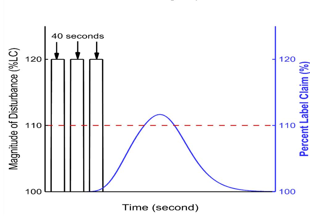
**Description:** Figure 8 illustrates a drug substance LIWF with multiple frequent transient +20% flow spikes, each lasting 40 seconds, resulting in variability in the amount of material fed into the blender.
