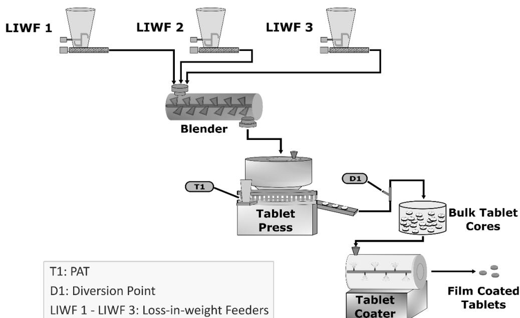
A PAT tool using an NIR method monitors blend uniformity and triggers tablet diversion. Run time at a predefined mass flow rate is used to define the batch size range; in this case, the overall marketing demand requires batch sizes between 360 and 1080 kg of the drug product.
