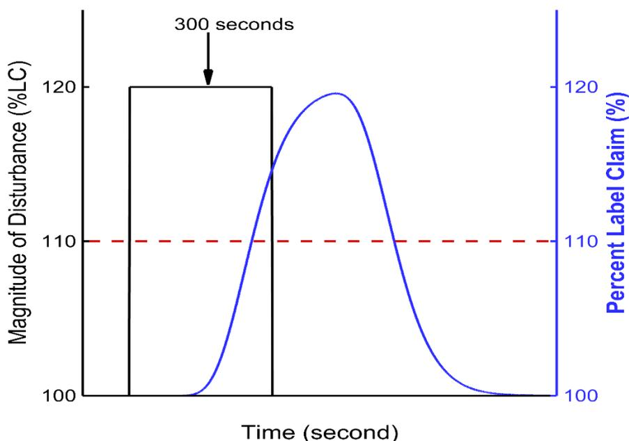
**Description:** Figure 7 illustrates a drug substance LIWF with an unexpected transient +20% flow spike lasting 300 seconds. The disturbance is outside the predefined acceptance criteria for disturbances. This disturbance causes an increase in the amount of the drug substance fed into the blender before returning to normal operating condition. The funnel plot (Figure 5) shows that following this disturbance, the drug substance concentration in the blend exceeds the 90–110%
